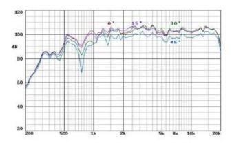
Notes: dispersion measured with two waveguides coupled to a 80° x 5° horn in anechoic chamber, 1w@ 2m.
