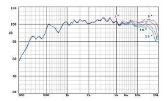
**Notes**: dispersion measured with two waveguides coupled to a 80° x 5° horn in anechoic chamber, 1w@ 2m. All angle measurements are from the axis (45° means + 45°).
