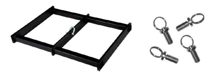
**Rigging Hardware frame for GTA 2X12 L.A. composed by:** one (1) lightweight steel frame+ four (4) pinlock + one (1) shackle to support a maximum weight of two (2) tons. It can elevate up a total of 16 GTA 2X12 L.A.
