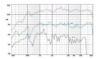
**Note**: on axis frequency response measured with 2 waveguides coupled to a  $80^{\circ}$  X  $5^{\circ}$  horn in an anechoic chamber, 1 w@ 1 m.
