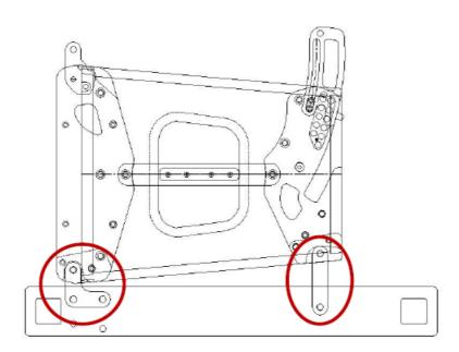
If the array is stacked on a subwoofer, it will be necessary to secure it by using slings. In any case, it is not recommended to stack more than 6 AVIATOR LA 212 A units.
