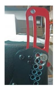
3. Install the fly bar to the box using the fixation pin locks.
