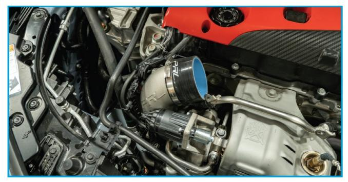
12. Install the new PRL Inlet Pipe into the elbow as shown below, aligning the rubber grommet with the factory mounting standoff next to the valve cover.
