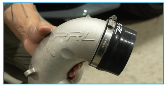
10. Make sure the surface of the Inlet Elbow that mounts to the turbo is clean and clear of any debris. Install the factory gasket onto this surface with the tabs wrapping around the flange as shows below.
