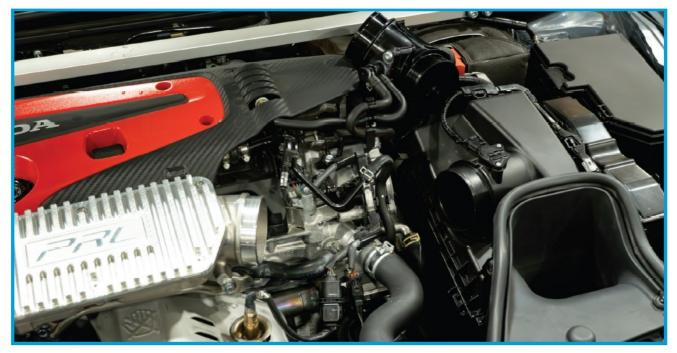
4. Remove the two 10mm bolts securing the upper turbocharger coolant feed line to the underside of the factory aluminum inlet pipe.
