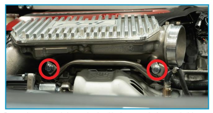
5. Remove the two 10mm bolts securing the wiring harness to the factory turbo inlet.
