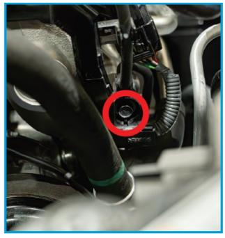
Disconnect the connect on the turbocharger wastegate motor and pull back the wiring harness to allow enough room to maneuver the factory turbo inlet out of the engine bay.
