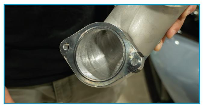
11. Install the PRL elbow onto the turbo in place of the factory inlet. Ensure that the wiring harness and bracket run on the outside of the elbow, similar to how they were oriented with the factory inlet. Reuse both of the factory bolts you removed in step 7. Torque both bolts to 8 it-lbs.
