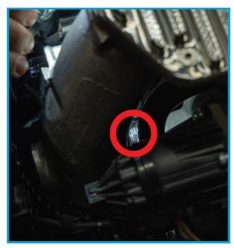
8. Remove the rubber grommet and steel sleeve from the factory inlet and install them as shown on your PRL Titanium Inlet pipe. Quick tip: If the sleeve is stuck inside of the grommet on the factory inlet, you can gently pry it out with a flat head screwdriver.
