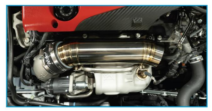
13. Install both of the other couplers in your kit onto the inlet pipe as shown below. Make sure to orient the shorter silicone coupler to the breather hose connection.
