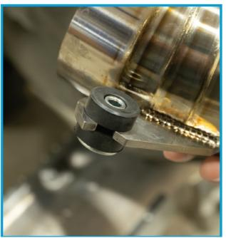
9. Loosely install the shortest coupler of the three included in your kit onto the PRL Turbo Inlet elbow as shown below with the wider side on the machined lip of the elbow. Now is a good time to install one of the larger worm clamps from your kit on this joint as well.
