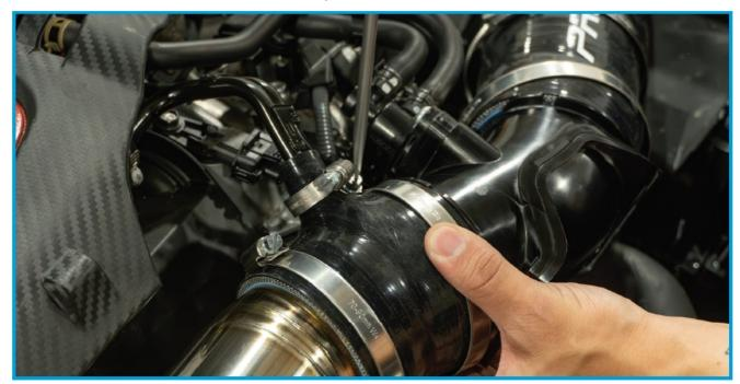
14. Securely tighten all the worm clamps. Once done, reinstall the two 10mm upper turbocharger cool- ant feed line bolts you removed in step #4.
