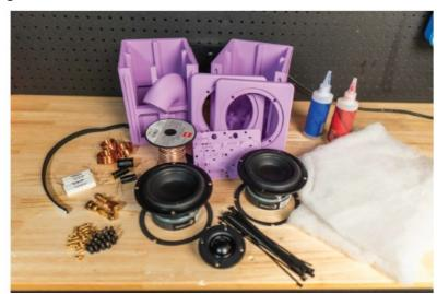
• Lay It Out: Pop those components on the crossover board, right where they need to be based on their values. Thread those wires through the wire holes, don't skimp on the hot glue and cable ties to keep everything snug as a bug. Snip the cable ties to prevent them from rattling inside the speaker.
