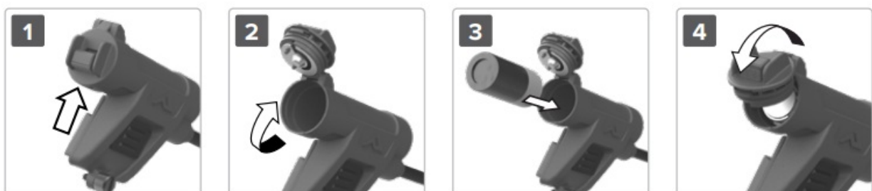
Figure 1 – Battery Installation
