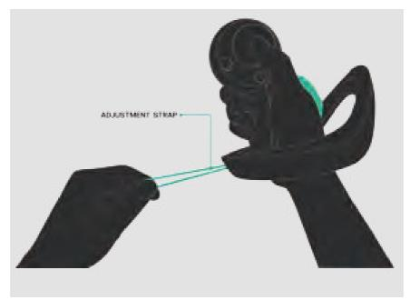
Hold the Controller with your hand and pull the strap to fix it (the handle will not fall off when the palm Is opened).
