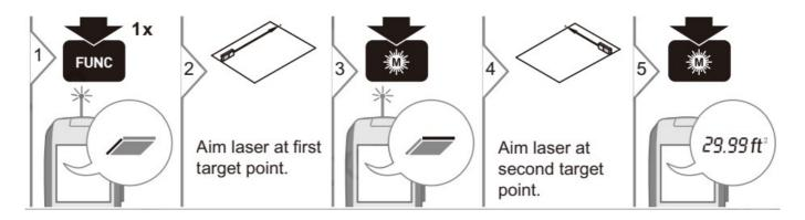
i The result is shown in the main line and the measured distance above.
