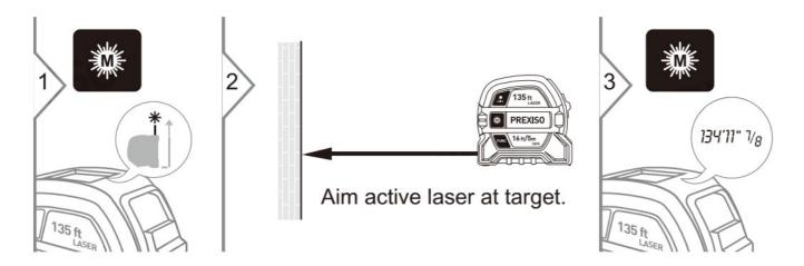
i Target surfaces: Measuring errors can occur when measuring to colourless liquids, glass, styrofoam, or semipermeable surfaces or when aiming at hight gloss surfaces. Against dark surfaces, the measuring time increases.
