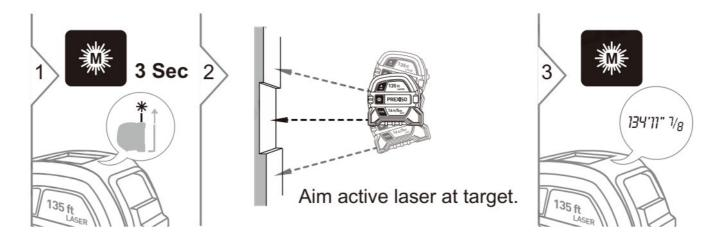
i Target surfaces: Troubleshooting can occur when measuring to colourless liquids, glass, styrofoam, or semipermeable surfaces or when aiming at high gloss surfaces. Against dark surfaces, the measuring time increases.
