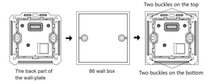
**Step 2:** Align the front part of the wall-plate with the socket at the rear of the wall-plate, then press the Force Point 1 and Force Point 2 (see the figure below) perpendicular to the wall at the same time, until the two buckles on the top are fully buckled.
