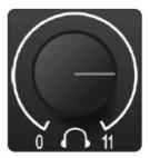
This knob controls the level of the rear panel headphone output.
