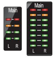
These meters display the signal level received from the first two driver returns (Main Left/Right). These meters have the same range as the input meters and display the signal level before the main output level control.
