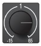
These knobs adjust the gain for your audio interface inputs.
