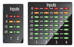
These LED meters show the input level of the analog inputs on your Studio-series interface. The red Clip LED will illuminate when your input signal reaches -0.5 dBFS. At this level, the signal will begin to overload the analog-to-digital converters and exhibit signs of clipping. Use the gain controls to keep the signal below this level.
