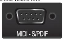
This is where you connect the breakout cable for the MIDI and S/PDIF I/O.
