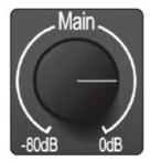
The main knob controls the output level for the main left/right outputs on the back of your Studio-series interface and has a range of -80 dB to 0 dB. This control provides attenuation only.
