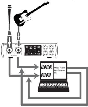
When Loopback is enabled and "Virtual" is selected in Universal Control, the audio from another application will be recorded on the last pair of driver inputs (Studio 26c: 5/6, Studio 68c: 7/8).
