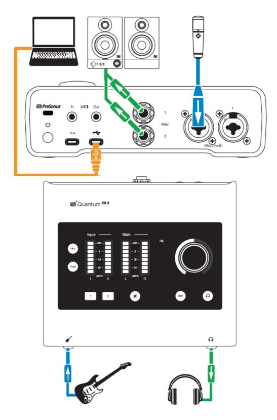
**Note**: Using the front Instrument Input disables Input 1 on the rear panel. Unplug from the front panel to access the back panel Input 1.
