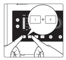
After 10 seconds, the knob (cap) will blink green 3 times if successful, then the knob and ring will return to white again, showing the new gain position. If Auto Gain cannot determine the best level, the knob (cap) will blink red 3 times and the knob will return to the last known gain level position (white).
