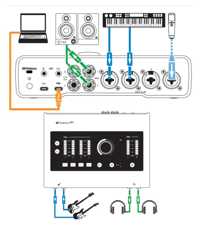
**Note**: Using the front Instrument Inputs disables the corresponding inputs on the rear panel. Unplug from the front panel to access back panel Inputs 1 & 2.
