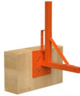
Parapet Installation with eight (8) 3/8" x 2-1/2" Lag Screw
