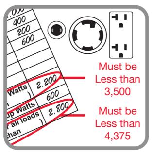
Check total Start-up watts amount before plugging in any equipment. To check the wattage amount:
