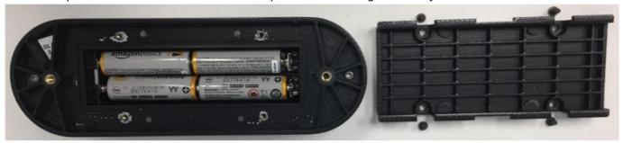
Install the four AA batteries as shown below. Note: The SFD1000 has protection to prevent damage should the four batteries be installed backwards.
