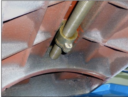
Figure 4-4 Y-axis backlash adjustment
