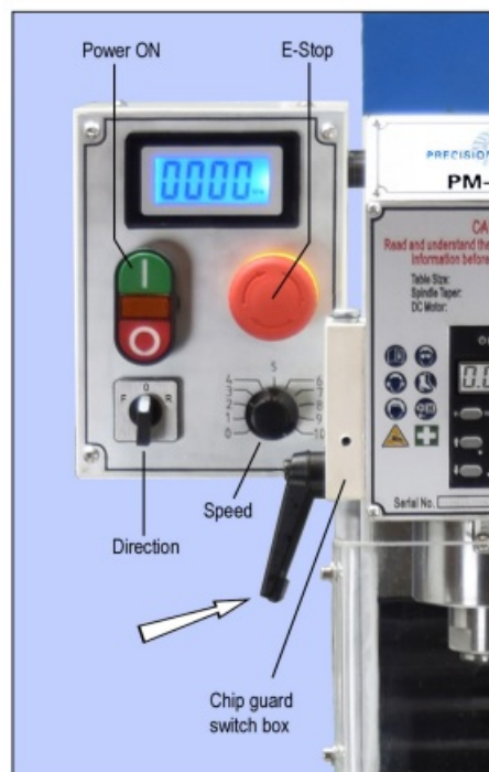
Figure 3-1 Spindle motor controls Also shown, arrowed, is the quill locking lever
