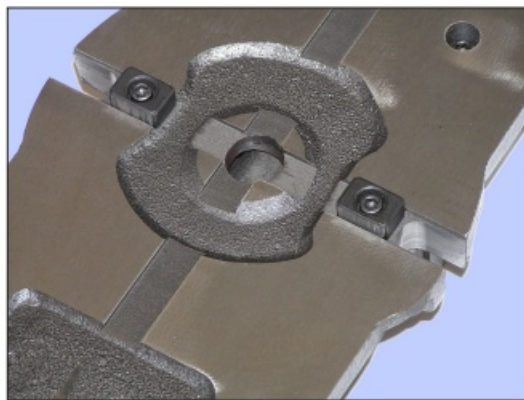
Figure 3-14 Vise keys installed on X-axis On most vises the keys can also be installed on the long axis.
