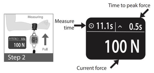
**Step 3** – Stop measurement either by pressing themain button or instruct the patient to stop pulling. When the force drops below 1 N the measurement will automatically stop.
