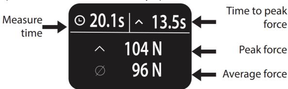
**Step 4** – To save the measurement and return to the history view, press the main button. Alternatively, press the delete button to return to the history view without saving.
