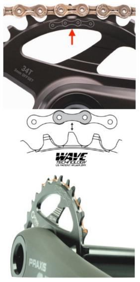
**CHAIN INSTALLATION:** Using the icon on your Wave Ring, Make sure your chain is aligned and placed correctly on the Wave Tech ring or chain will not sit down and ride on teeth correctly.
