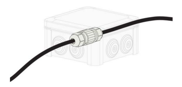
Make the connection inside the box using a waterproof connector (min IP67).
