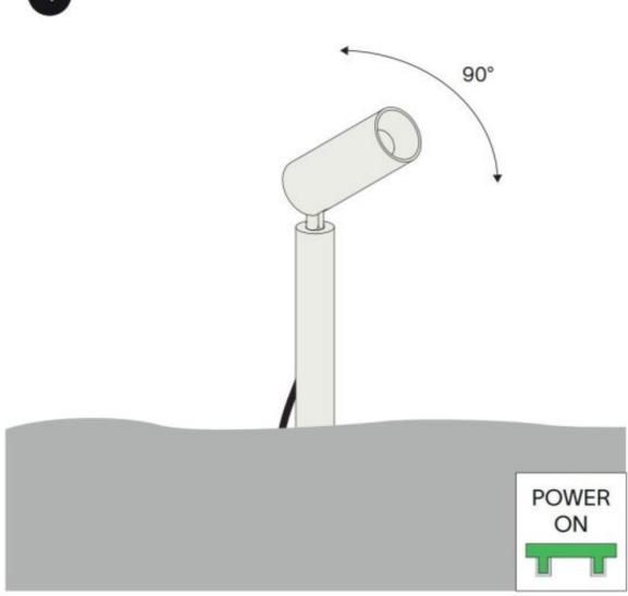
Twist the fixture as desired and turn the power back on.
