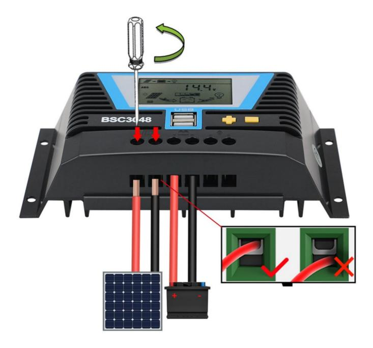
**NOTE:** This controller only charge battery when Solar panel voltage higher than battery voltage. Please make sure PV voltage is higher than battery voltage.
