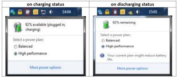
• You can set to Sleep/Hibernate/Shutdown OS or do nothing when it reached Battery Low Level or Battery Critical Level (with OS without Winpower).
