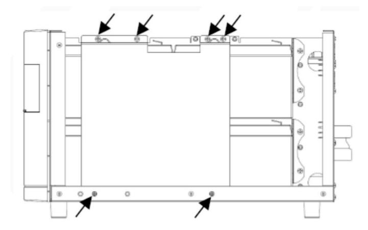
Step 7: Put metal top cover back to the unit and secure it with screws.
