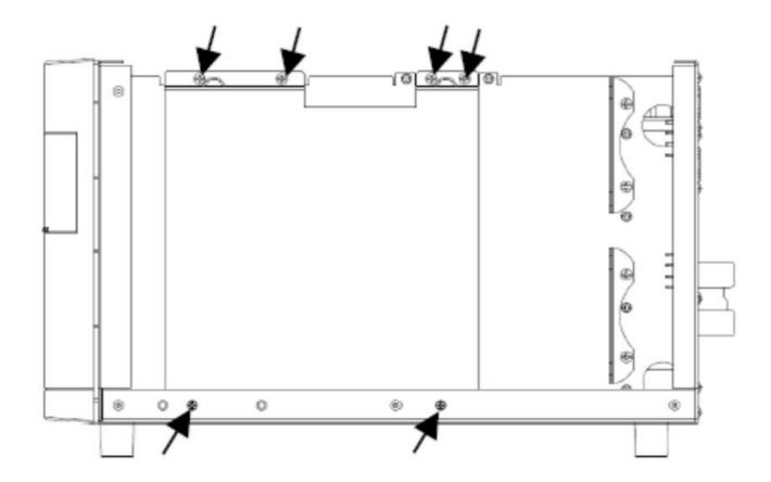
Step 4: Now, it is possible to put all batteries in battery pack following the picture below (in the following drawing is indicated the fasten positions for the correct batteries placing).
