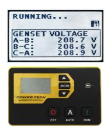
\* **NOTE:** The genset mounted controller must be in "AUTO" mode in order to enable the remote panel functionality.
