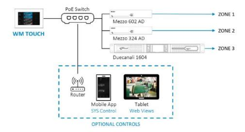
A PoE injector or PoE switch is necessary for powering the WM Touch and a regular Cat5 cable (or above) can be used for connection. The WM Touch must always be in the same network that is connected to the control ethernet ports of the amplifiers, as indicated below.
