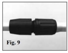
• Unscrew the lock sleeve on the shaft and adjust the length of the telescopic shaft (K) to the most comfortable operation position. See fig 9. Turn the lock sleeve anti-clockwise to lock the shaft in position.
