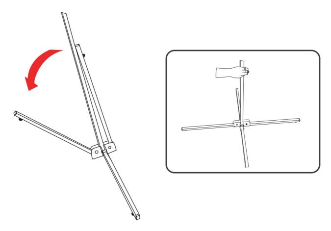
2. Insert the **Dual Pole Holder** into the **Base Frame.** Push in the silver button until the bottom hole is reached on the **Base Frame.**
