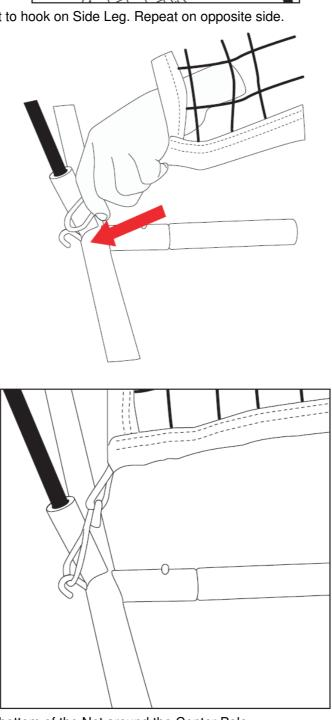
6. Attach red securing flap on bottom of the Net around the Center Pole.
