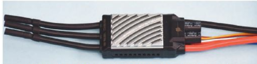
A close-up of the iESC showing the nicely machined heatsink and filter capacitors
