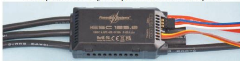
Underside of the iESC, where the connection for the (blue, red and white) telemetry lead and main throttle channel lead can be seen
