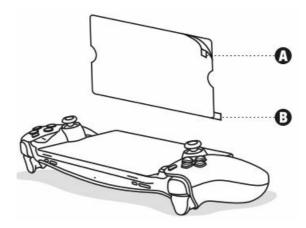
2. Apply the screen protector from the edge of the screen. Use the applicator included to remove any bubbles.
