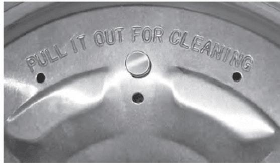
For proper cleaning the Rubber Gasket should be removed. Using the Pull Tab located beneath the Lid, remove the Pot Lid Liner that holds the Gasket. After cleaning, re-attach Gasket to Lid Liner and snap back in place.
