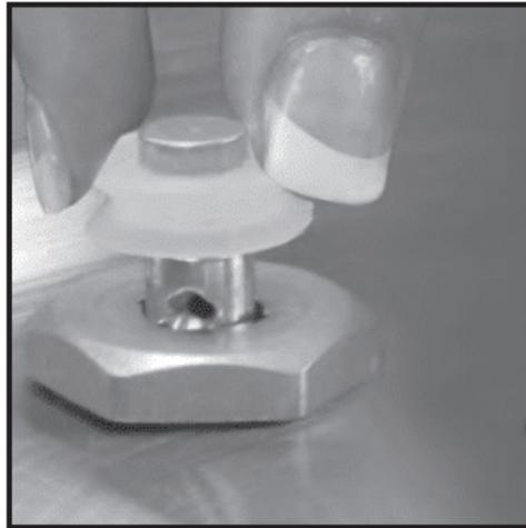
4. The Float Valve should be able to move up and down freely only stopping when the silicon gasket meets the Lid.
