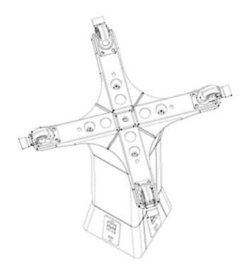
Note: AC-COLLABR-8TM has low center of gravity which provides stability when moving and avoids tipping.
