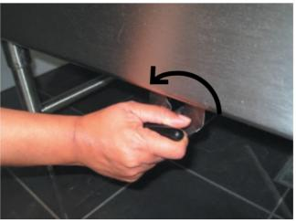
Remove each Power Prep Intro component (flow guides, partitions, and rib sets) in the reverse order they were assembled. Wash each component to remove all traces of produced debris. Position each component so that it dries quickly. Pay particular attention to the flow guides; provide airflow between each of them and do not stack them together wet.
