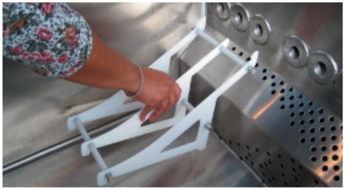
Place the other rear rib sets against the back wall of the sink leaving a finger-size gap between them.
