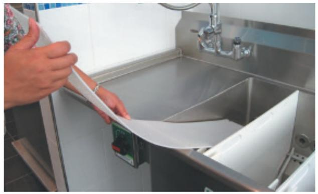
Begin bending the flow guide to the shape of the front rib set, and allow the notches of the flow guide to engaging the hooks of the rear rib set.
