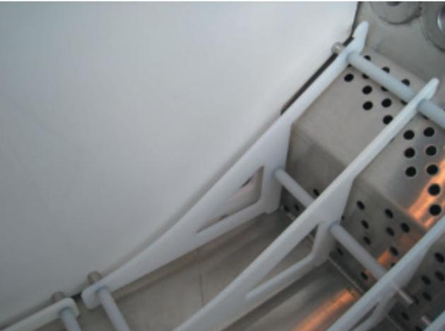
Continue until all three partitions are in place. It will be necessary to push all previously placed components together to make room for the final partition.
