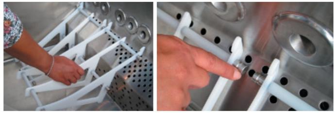
When you have placed all of the rear rib sets, begin placing the front rib sets against the front wall of the sink. As with the rear rib sets, place the first front rib set against a corner, and leave a finger-size gap between it and the next front rib set.
