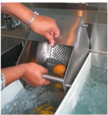
Rest the basket on the top edges of the partitions or the sink edges until all the produce is collected. Lift the full basket out when ready. Always observe safe lifting procedures.
