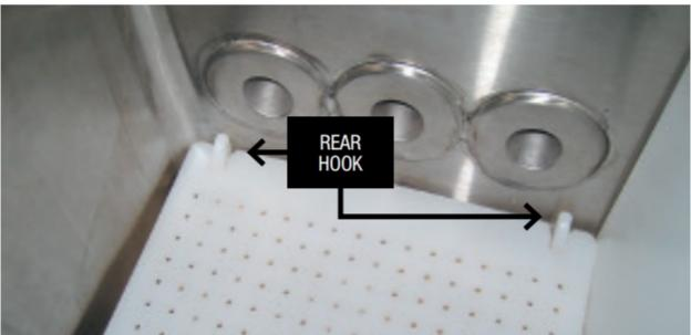
Continue to push the flow guide down against the rib sets until the notched end of the flow guide nearest you is adjacent to the hooks of the front rib set.
