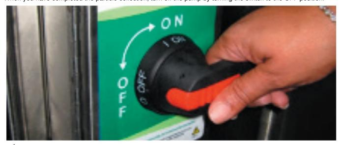
DO NOT RUN THE MOTOR WITHOUT WATER IN THE SINK. DOING SO COULD DAMAGE THE SEALS IN THE PUMP.
