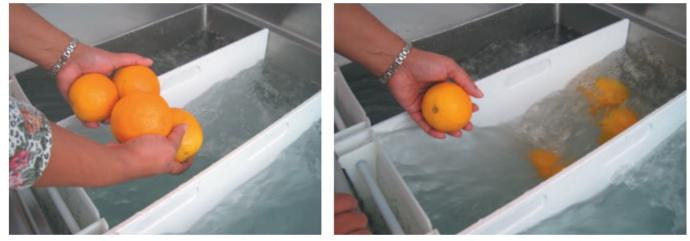
After the necessary time for soil removal and disinfection, the product may be removed by inserting a collection basket. Holding the basket as shown, angle the basket so its leading edge is aligned with the flow in the sink. As you swing the basket into position, production will begin flowing into the basket.
