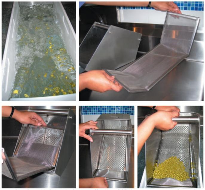
Allow a few minutes of collection time in each position. When finished, empty the contents of the filter into a suitable waste container, and wash out the filter and basket.
