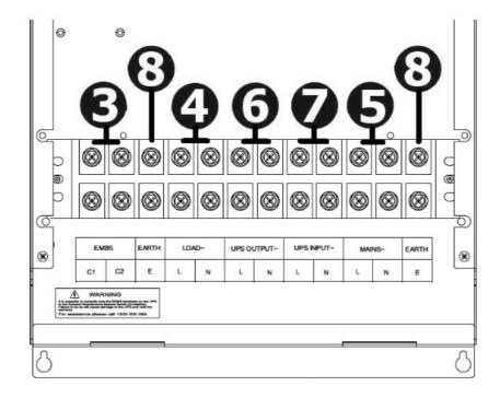
**WARNING**: It is essential to connect the EMBS (C1, C2) terminals on the UPS to the EMBS (C1, C2) terminal on the Maintenance Bypass Switch module. Failure to do so will cause damage to the UPS and void the warranty. Check the UPS model User manual for the Rear Panel Terminal Block Pin assignment.
