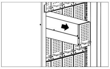
4. Remove the empty battery module cover.
