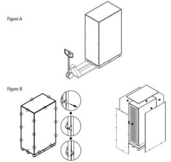
(3) The four sides of the battery cabinet feet are fixed with screws and nuts. Loosen the screws and nuts to remove the fixing on the cabinet and pallet. Refer to figure below.
