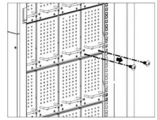
3. Remove the empty battery module.
