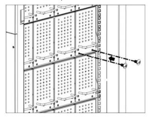
7. Insert the battery module back into the battery cabinet.
