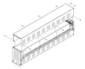
5. Assemble the 9AH 12V battery into the empty battery module, as shown below.
