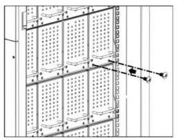
9. Starting from the bottom, install all battery modules.
