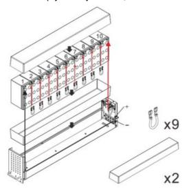
6. Assemble the top cover and lock the screws in sequence.
