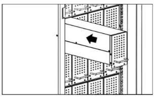
8. Fasten screws to lock the battery modules.
