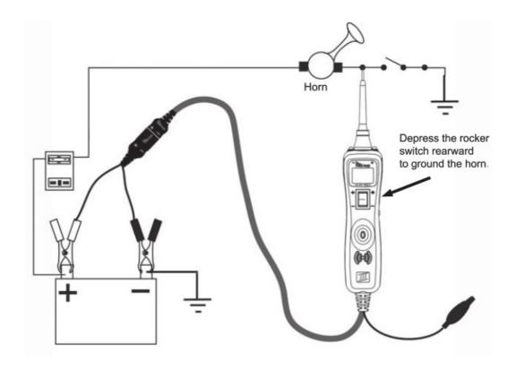
**WARNING:** With this function, if you are contacting a protected circuit, a vehicle's fuse can be blown or tripped if you apply ground to it.
