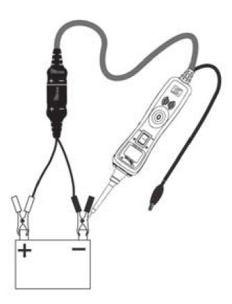
While the PP3 is in Power Probe Mode. Contact the probe tip to a NEGATIVE circuit. The green negative sign "-" LED will light. If the audio feature is turned on, a low pitched tone will sound.
