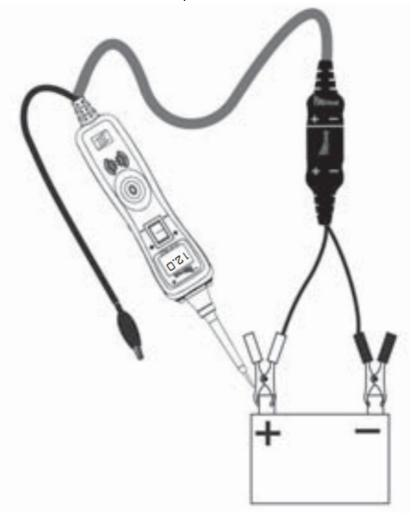
While the PP3 is in Power Probe Mode, contact the probe tip to a POSITIVE circuit. The red positive sign "+" LED will light and the voltage reading of the circuit will be indicated on the LCD display. If the audio feature is turned on, a high pitched tone will sound.
