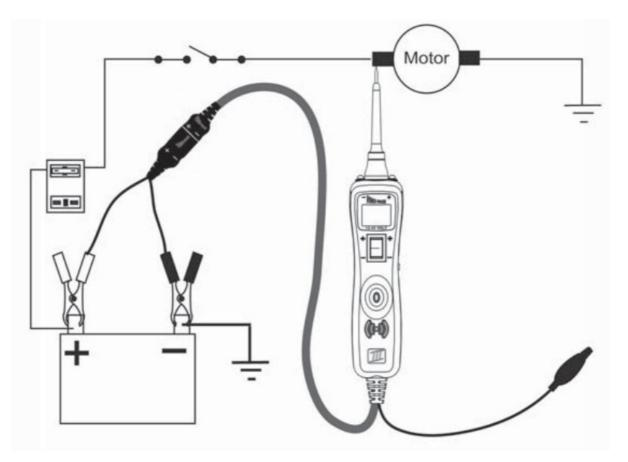
**TRICK:** When poweringup components, you can increase the life of your Power Probe switch if you first press the switch, then contact the tip to the component. The arcing will take place at the tip instead of the contacts of the switch.
