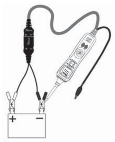
While the PP3 is in Power Probe Mode. Contact the probe tip to a NEGATIVE circuit. The green negative sign "" LED will light. If the audio feature is turned on, a low pitched tone will sound.
