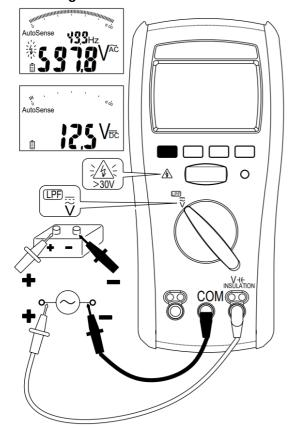
Auto sense mode: The meter displays ACV or DCV whichever is higher (>1V).
