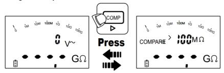
Before starting the Insulation Resistance test, select the comparative value in Setup mode:  $0.5M\Omega$ ,  $10M\Omega$ ,  $20M\Omega$ ,  $50M\Omega$ ,  $100M\Omega$ ,  $200M\Omega$ ,  $1000M\Omega$ ,  $1000M\Omega$ .
