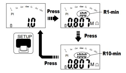
Show the measured values after the DAR test is completed
