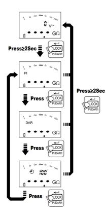
Press TEST button to start/interrupt the PI/DAR test. Press Function button during the PI/DAR test to switch display the output voltage / leakage current / the time left of the test.
