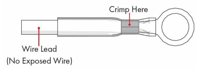
**IMPORTANT!** Check Ring Terminal or Butt Connector for any cuts from crimping and give the cables a slight tug to ensure they are properly crimped. Poorly crimped or damaged connectors will not provide a water-tight seal. This will lead to corrosion and wire failure.
