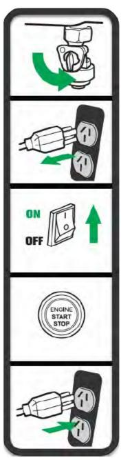
6. **ELECTRIC START** – press the engine start button or use the wireless starter fob. The engine should fire in less than 5 seconds.
