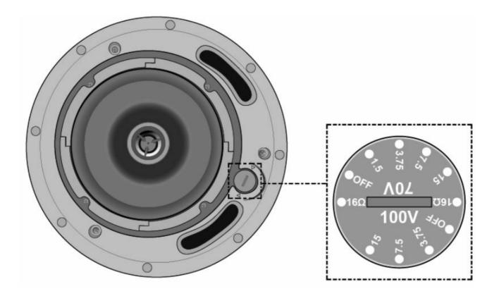
Before connecting, always make sure to set the rotary switch to the correct position! Never set the switch to "empty" position for 100V line operation, as doing so may result in unrepairable damage.
