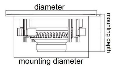
This speaker for ceiling mounting is a 100 Volt system specially designed for application in PA systems and must only be used for permanent installations, to be connected with an appropriate 100V-amplifier.
