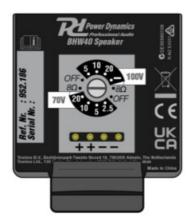
The BHW series speaker is functional both in low impedance-, as well as in 100V/70V use. Use the rotary switch (pictured) to set the speaker in the correct working mode. In below case, the speaker is configured to work in 8 Ohm ( $\Omega$ , low impedance) setup.
