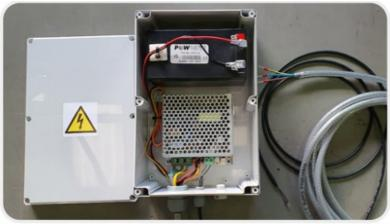
Ideally a flat surface such as a wall/ DIN railing/ \Unistrut railing. Avoid mounting inside metal cabinets or \underground (could reduce signal). We supply a 2m cable to connect the UPS to the Metron5. It is OK to trim to suit the installation.
