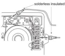
**Step 4**Connect the siren and strobe wires to the terminal strip as indicated above.
