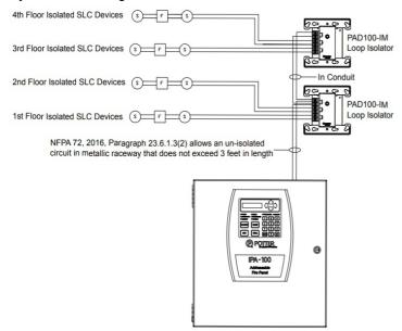
Class B wiring example using IPA series fire alarm control panel and PAD100-IM loop isolation modules.
