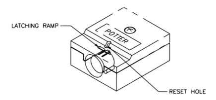
To unlatch the HUB-M, insert a small pointed object, such as a pocket screwdriver or paper clip into the reset hole. The unit unlatches when the cap is released.
