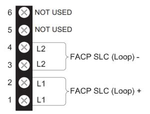
**SAMPLE CONTROL PANEL WIRING – STYLE "6" / "7" SLC** (Supervised – A single open/ground condition will not inhibit an alarm response)
