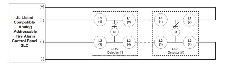
**SAMPLE CONTROL PANEL WIRING – STYLE "4" SLC** (Supervised – A single open condition will inhibit an alarm response)
