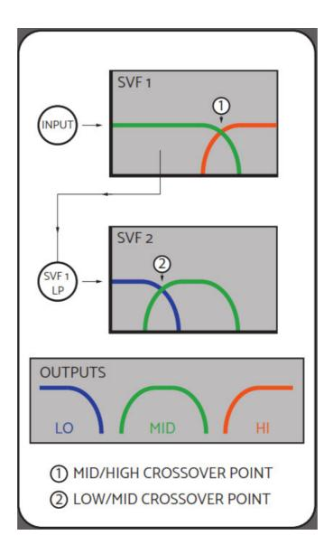
The LR4 Crossover comprises two state-variable filters in series. The high-pass from the first SVF gives the HI output, while the low-pass serves as the input to the second SVF. The high-pass of the second SVF gives the MID output, and the low-pass the LO output.
