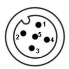
Connect the shield of the cable to the connector housing for proper EMC shielding measures. It is not recommended to connect the shield to CAN Ground.
