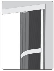
6. Start the installation of the mosquito net package from inserting the bottom part of the profile into the protruding
