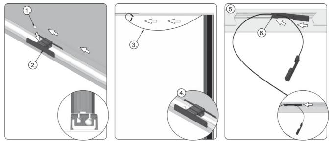
7. Stretch the bottom cords of the mosquito net. Make sure they do not get entangled, twisted or bundled. Put cord ends (1) in the cord lock of the bottom rail (2). Stretch the upper cord (3) so that the bottom cord gets properly tensioned and blocked (4). Properly place the upper cords. Pay particular attention and make sure that they are not entangled, twisted or bundled. As shown in figure 5, slide the element of the cord lock (6) through the milled hole in the upper rail in such a manner...
