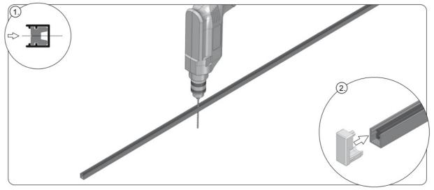
4. Drill the mounting holes in the lateral profile of the mosquito net through the profile and the magnet (1), using the 3.5 drill bit.
