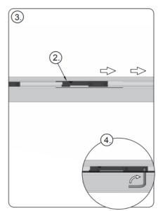
9. Insert the second lock (2) in the same milled hole (1) in the upper rail, slide the lock in the direction opposite to the first lock (3), this way, you will stretch the mosquito net cords. Fix the lock by tightening the socket head screws (4).
