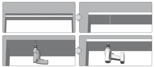
2. Fit the upper slat of the mosquito net in the upper recess of the door opening, mark and drill holes for the screw anchors.
