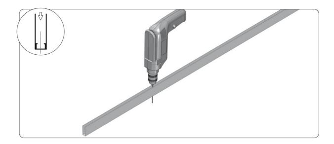
1. Using the 4.2 drill bit, drill the mounting holes in the upper rail of the mosquito net. The holes shall be drilled at every 50 cm and there shall be at least 3 holes in each profile.
