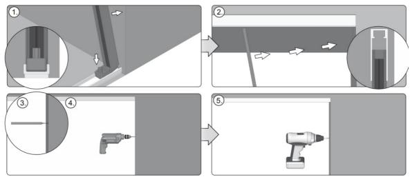
5. First, insert the lateral profile ended with the end cap in the bottom slat (1) by sliding the end cap into the slat, next slide the profile towards the mounting frame at the recess side, make sure that the upper part of the lateral profile gets fitted into the upper profile (2).
