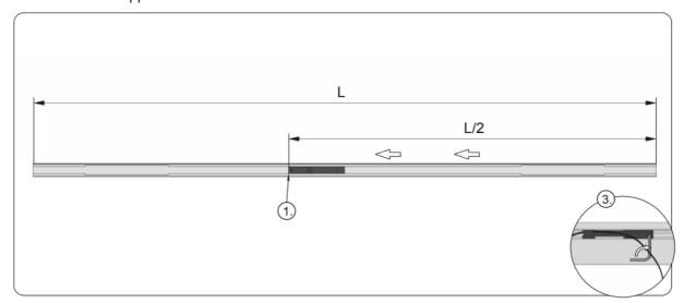
8. that the lock end (1) is exactly in the middle of the upper rail. Fix the lock by tightening the socket head screws (2).
