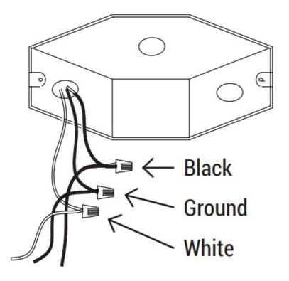
5. Arrange the wires into the Junction Box. Align appropriate slots in the disk light with the holes in the Junction Box. Use 2 screws to attach the disk light, flush with the ceiling
