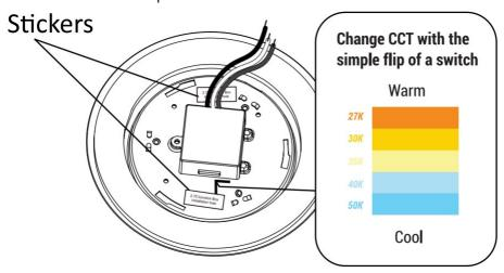
4. Connect the supply wires to the wires of disk light by using 3 wire nuts. Attach white to white, black to black, green to the ground wire.
