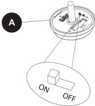
The power switch, located on the back of the solar panel, has 2 settings-ON and OFF. Push the switch to the "ON" position to allow the path light to automatically turn on at dusk. If you do not intend to use the path light for an extended period of time, be sure to move the switch to the "OFF" position.
