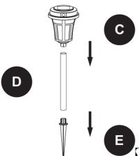
Attach lens (C) and ground stake (E) to pole (D). Then, apply pressure to the pole (NOT
